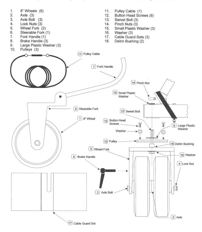
1. Slide the Wheels onto the Axle.
