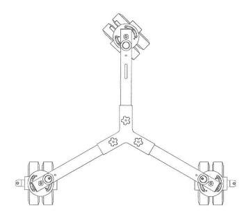
If you want to maneuver the Dolly by steering with the leading wheel it will be necessary to lock the two back wheels. This is accomplished by inserting two spacers into the pulley slot and inserting two screws through the Dolly Leg into the fork.
