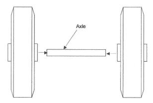
2. Insert the Wheels and Axle between the Forks and secure with the Axle Bolt.
