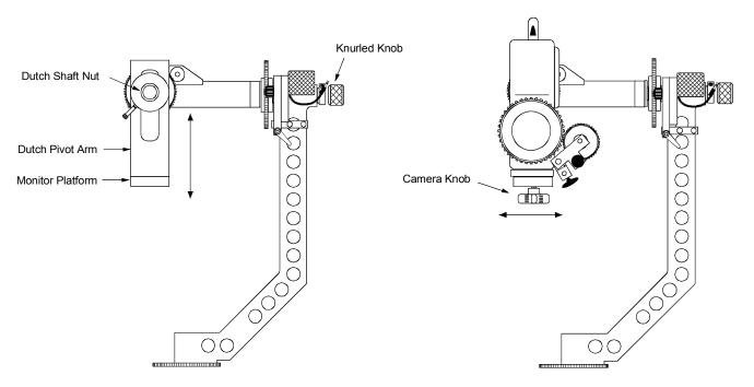
Once the camera is completely balanced you should be able to rotate and tilt the camera into any position and it should remain in that position.
