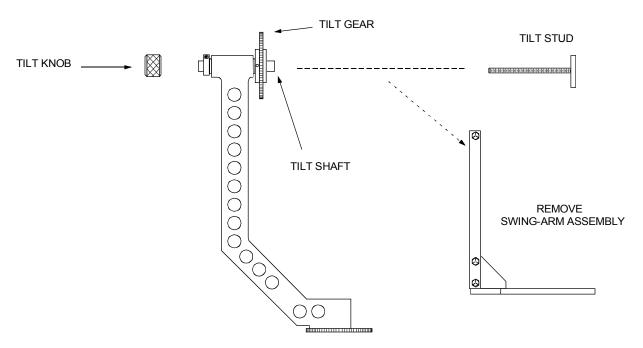
2. Install the Dutch Axis Assembly in place of the Swing Arm and attach using the Tilt Stud and Tilt Knob.
