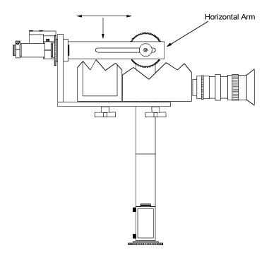
2: <u>Vertical Balance:</u> Loosen the large circular Dutch Shaft Nut so that the Dutch Pivot Arm can moved vertically. Slide the camera vertically until it is in balance. It may also be necessary to slide the camera sideways using the slots in the camera platform.
