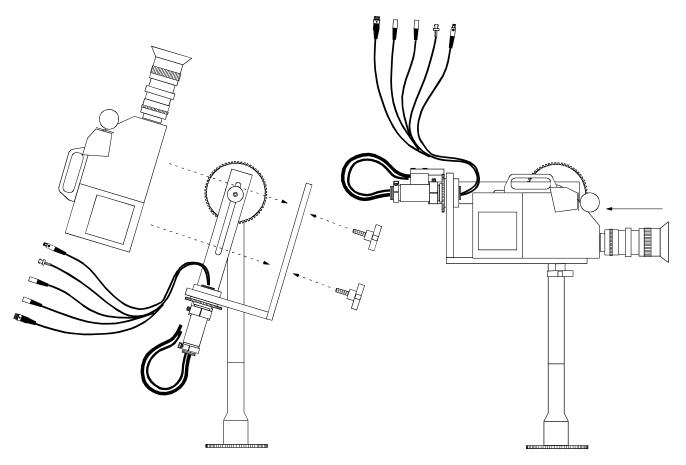
5: The Iris and Focus servos should also be attached before you balance the camera.
