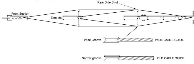
6. Before adjusting the cables you must counter weight the jib with at least 200 lbs.
