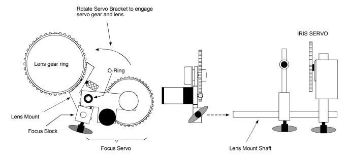
If you have a Canon Lens, the Master Gear will directly engage the lens. If you have another lens it will be necessary to add an extra gear. Slip the extra gear over the hub of the Master Gear and secure with the 4-40 screw.
