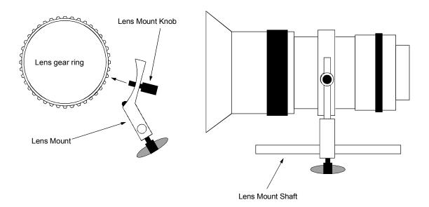
Occasionally the curvature of this mount is greater than the lens curvature. This means that there will be contact only at the center of the mount instead of along the entire curve. This can cause the Focus/Iris assembly to twist on the lens. To correct this problem, adjust the set screw in the Lens Mount. Back out this set screw only far enough to just touch the lens.
