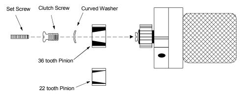
It has been found that the use of the small 22 tooth pinion on the <u>Tilt Axis</u> has improved the "feel" and movement of this Axis. This is especially true when using heavier film cameras. This small pinion is available as an accessory.
