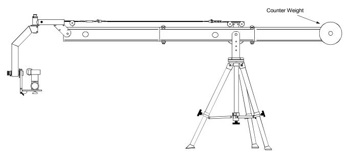
3. Start by loading 25 lb. plates on the weight bar, <u>stacking them equally on both sides of the Rear Tube</u> <u>Section.</u> Switch to lighter weights as the Jib becomes more balanced. When you get to within about 5 lbs. of the balance point, you may wish to fine tune the Jib with the optional sliding Ballast Bag.
