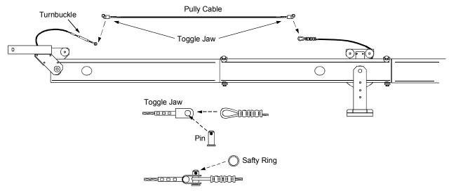
3. The Pulley Cable must be properly aligned with the Cable Spools.
