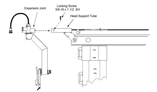
6. The Head can be leveled Sideways by loosening the Locking Screw and rotating the head to a vertical position.
