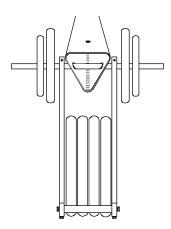
If you wish to place all the weights on the bottom bar the most compact configuration is to insert the second weight bar through the uprights and the weights as shown below. In order to accomplish the center holes of the plates must be in alignment.
